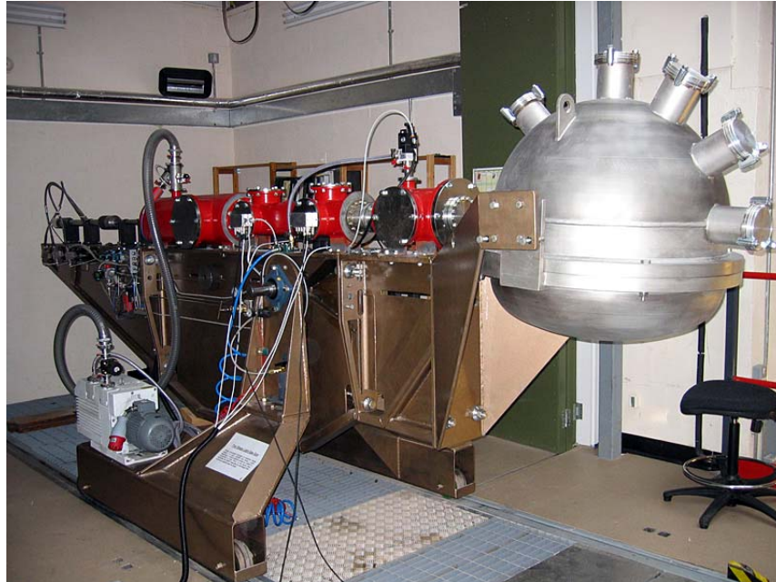
Figure 2-7: The all- axis light gas gun (shown here horizontally) installed at the Open University. In order to simulate vertical and oblique impacts, the entire assembly pivots to accommodate a range of angles.
