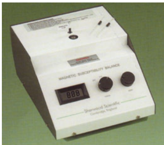
Figure 5-2: The Sherwood Scientific Magnetic Susceptibility Balance (MSB), Mark I. This instrument is an Evans balance and can accept solid or liquid samples as small as 50 mg.
