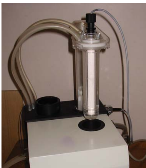
Figure 3-5: The KLY-3 susceptibility bridge with CS-2 furnace at the University of Birmingham. The furnace is shown during the bridge zeroing part of the measurement cycle.
