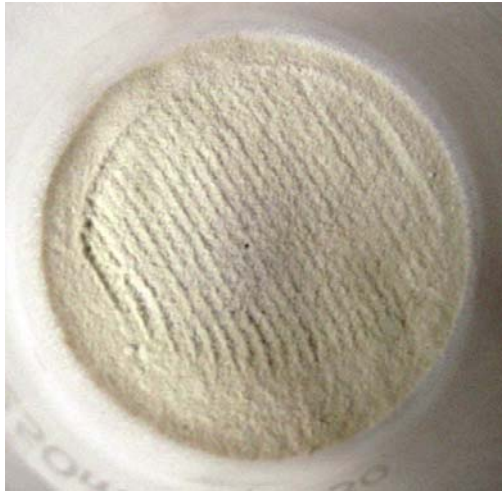
Figure 3-2: An example of the visible pattern left after a sample has been irradiated. The scan pattern visible here has a diameter of 54 mm.
