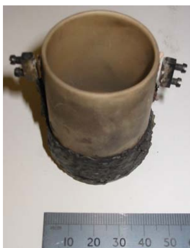
Figure 2-19: The heater pot, after a period of use. The lower portion is covered in heater cement to support the heater wire windings.
